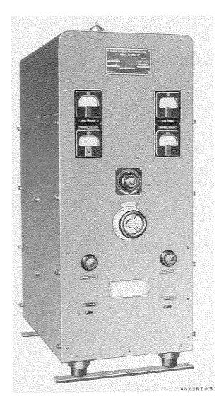
Radio Transmitting Set AN/SRT-3 is a mediumpower, medium-range, crystal-controlled a-m (cw and mcw) transmitting equipment for ship-toship and ship-to-shore communication in the intermediate-frequency range.
