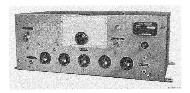
Radio Receiver R-215/SR is a medium-range, a-m (cw and mcw) receiving equipment which operates in the very-low-, low-, and medium-frequency ranges in shipboard or equivalent communication applications.
