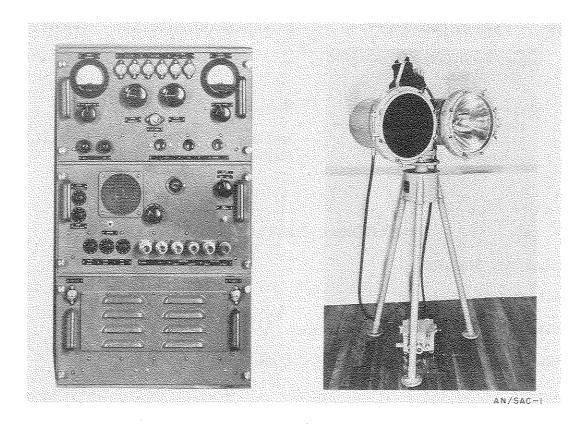
Infrared Communication Set AN/SAC-1 is a transmitting-receiving equipment for use at night during periods of radio silence in effecting a-m (voice, cw) soundless, invisible communication between ships by means of a beam of invisible infrared light.
