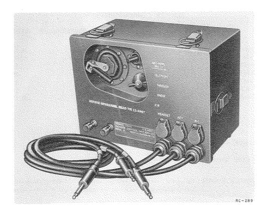
Remote Control Equipment RC-289 is an assemblage of items enabling the erection of a local battery telephone facility between a remote operating position and the actual site of the radio equipment. It is used in conjunction with radio equipment organic to company level units.
