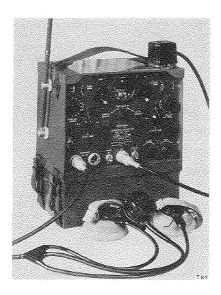
Ultra Portable Transmitting and Receiving Equipments TBY, TBY-1 and -2 are field, v-h-f radio communication sets designed for transportation as knapsack loads and may be operated while being carried on the operator's back.
