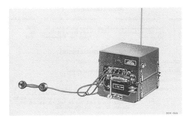
Radio Set SCR-509 is a portable, short-range, low-power, f-m (voice only), radio receiving and transmitting equipment used by armored, field artillery, and infantry units. The set is designed for operation on the ground but can be installed in a vehicle.
