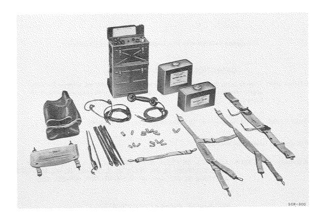
Radio Set SCR-300 is a portable, short-range, low-power, f-m (voice) transmitting and receiving equipment used for communication by foot troops at company and higher combat levels.
