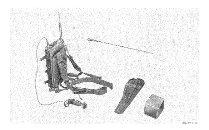
Radio Set AN/PRC-8 is a portable (man-carried), low-power, f-m (voice), radio transmitting and receiving equipment used for v-h-f, short-range, point-to-point, or radio relay communication by company and battery level units operating in the frequency range assigned to armored divisions. It can also be installed in aircraft.
