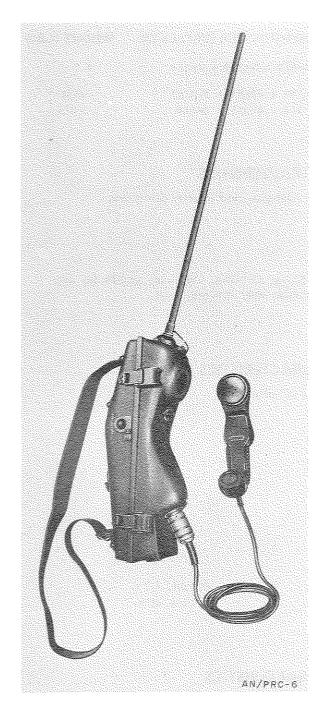
Radio Set AN/PRC-6 is the f-m version of the 'handie-talkie' Radio Set SCR-536 and operates in a single, fixed-frequency channel selected by use of the appropriate crystal. This is low-power, short-range equipment which operates in the v-h-f range for line-of-sight communication by forward elements of armored, infantry, and artillery units.
