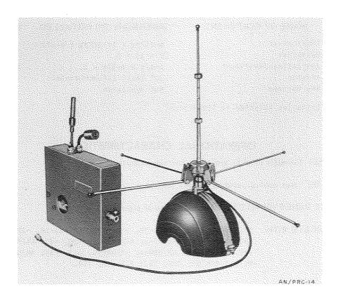
Radio Set AN/PRC-14 is a portable, a-m and c-w transceiver for point-to-point and ground-to-air communication in the u-h-f range 225 to 400 mc. This equipment is designed to be man-carried and can be operated, while in motion.
