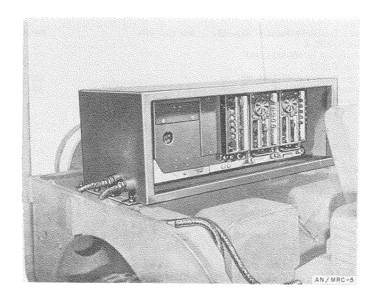
Radio Sets AN/MRC-5, -5A, and -5B are mobile, field, f-m (voice) equipment used in internal security applications. Each set is mounted on a 1/4-ton truck (jeep) and consists primarily of a Radio Set SCR-608 or similar equipment, a submersible cabinet, a remote control unit and accessories.
