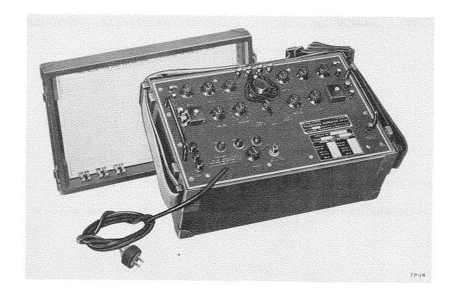
Telephone Repeater TP-14 is a portable, field, 22-type repeater equipment used to extend the range of two-wire (open wire or field cable) facilities which serve division or equivalent headquarters.
