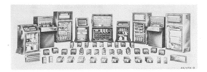
Telephone Central Group AN/GTA-3 is a complete telephone communication system used with, but not part of, Radar Set AN/FPS-3. It provides telephone communication between radar set operating personnel and outside points, which include aircraft in flight, radio communication with 12 v-h-f and three h-f transmitters and receivers, and wire telephone communication through four trunk lines to commercial telephone systems, with provisions for either magneto ringing or dial calling.
