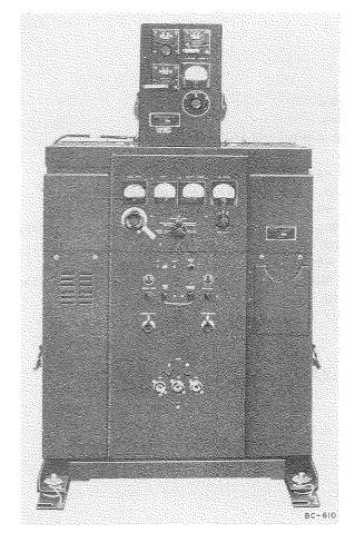
Radio Transmitter BC-610 is the widely used radio transmitting component of such equipments as Radio Sets SCR-399, SCR-499, and similar radio sets. It is a crystal-controlled or master oscillator a-m (voice or cw), medium- and high-frequency, radiotelephone and radiotelegraph equipment used in intermediate and long distance communication at division and higher headquarters.
