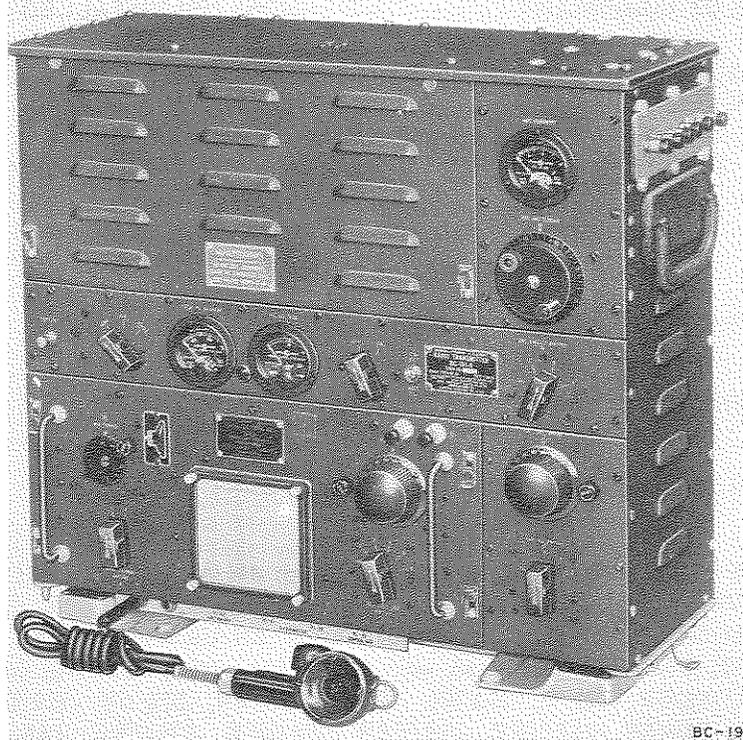
Radio Transmitter BC-191 is a general utility, medium-range, low-frequency, a-m (voice and cw) radio transmitting equipment which is widely used as part of Radio Sets SCR-177, SCR-188, SCR-193, and AN/VRC-1 and similar equipment. It can be used on the ground, in vehicles, and in aircraft and is used for ground-to-ground or ground-to-air communication.
