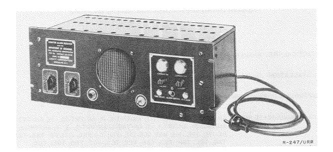
Radio Receiver R-247/URR is a rack-mounted, a-c operated, fixed-tuned, radio range, tuned-radio-frequency receiver designed for the monitoring of compass locator station transmitters. An alarm buzzer and signal lamps operate whenever the received signal drops below a predetermined level.
