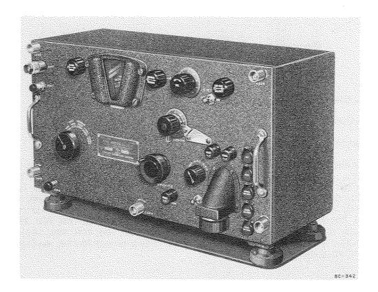
Radio Receiver BC-342 is a lightweight, a-m (voice, tone, and cw) receiving equipment which operates in the m-f and h-f bands and is the a-c operated equivalent of Radio Receiver BC-312. It is designed for general purpose ground, mobile, or fixed station use at division or higher headquarters.
