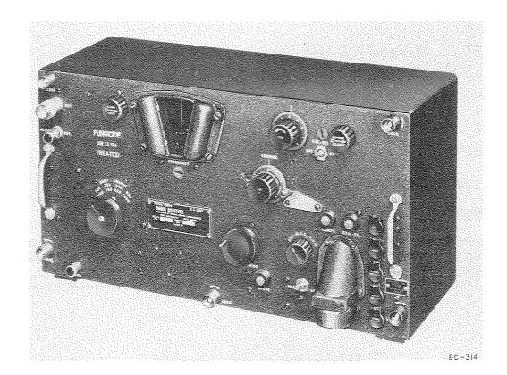
Radio Receiver BC-314 is a lightweight, portable, battery-operated, a-m radio receiving equipment used for voice, c-w, and tone signal communication in the l-f and m-f bands. It is a general purpose equipment which can be used in fixed station, mobile, or vehicular applications.
