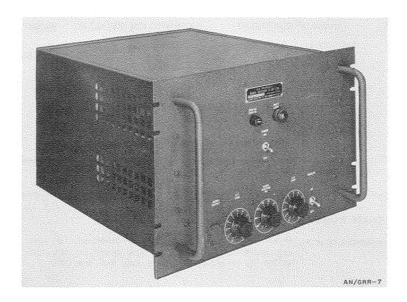
Radio Receiving Set AN/GRR-7 may be used for reception of a-m (voice or tone) signals in the u-h-f range 225 to 399.9 mc for general ground operation for air-to-ground and point-to-point communication. It is used primarily for control tower, and airway station operation, and has sufficient output to operate a loudspeaker.
