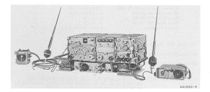
Radio Set AN/GRC-4 is a short-range, f-m (voice), two-way communication equipment having provision for retransmission, duplex, and remote control operation. It is one of the integrated series of radio equipment and is used by units organic to an armored division.
