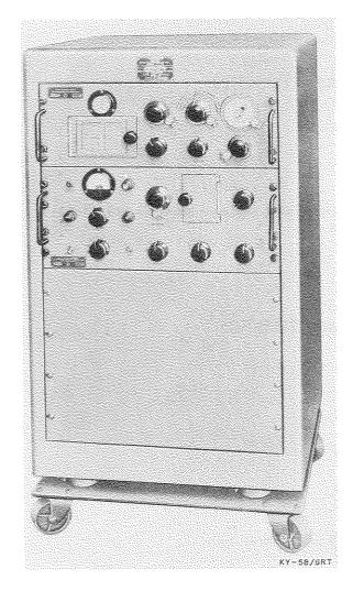
Keyer KY-58/GRT is used at long distance transmitting station to improve transmission. It replaces the exciter of a c-w transmitter, with a source of excitation that can be shifted in frequency (a small value higher and lower) to produce telegraph or facsimile signals corresponding to those delivered to the keyer input. This frequency-shift method is used to minimize selective fading, interference, and static disturbances.
