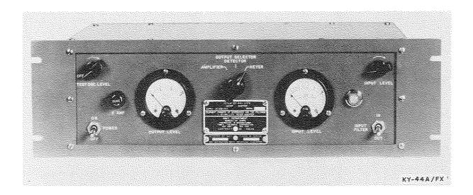
Keyer Adapter KY-44A/FX is used primarily for detecting and amplifying a-m facsimile signals and providing keying signals for frequency-shift exciter units in radio transmitter equipment. It can also be used as an unfiltered detector of a-m signals or as a line amplifier.
