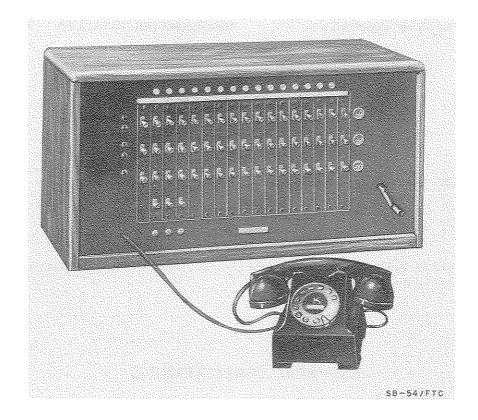
Switchboard SB-54/FTC is a cordless, manual, single-position, common-battery telephone switchboard used for establishing connections between a small number of local stations, or between such stations and a dial, or manual,central office. It is used in fixed-station applications in the communications zone of a theater of operations.
