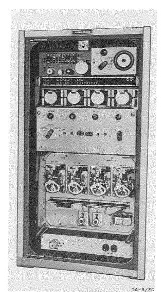
Regenerative Repeater OA-3/FC is an intermediate d-c, neutral only, repeater equipment used at points between two Telegraph Repeaters OA-6/FC in facilities serving army and higher headquarters.
