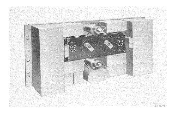
Carrier Repeater OA-10/FC is a single-channel, type H telephone and telegraph carrier-repeater equipment used to extend the range, in both directions, of transmission in a system operated in conjunction with Carrier Terminal OA-13/FC, or equivalent terminal apparatus. It is used at fixed station installations at army and higher headquarters.
