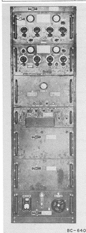
Radio Transmitter BC-640 is a 50-w crystal-controlled, a-m (voice or tone) v-h-f transmitter. Plug-in crystals are used to permit operation on any frequency in the 100 to 156 m-c range. It is normally operated from a fixed ground, or mobile location, for point-to-point or ground-to-air communication, and can be operated locally, or from a remote point up to eight miles away. The addition of repeater equipment extends the range of remote operation.
