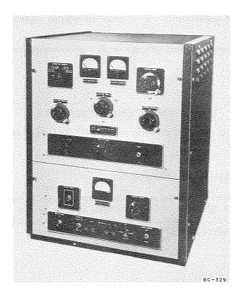
Radio Transmitter BC-329 is a fixed, ground, a-m radio transmitter for short-range airport control by voice communication in the 1-f (200 to 410 kc) range.
