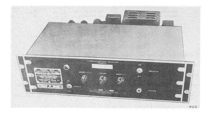
Radio Receiving Equipment RCO is a general purpose, crystal-controlled, fixed-tunes, single-channel receiver of modulated telegraph signals, and (more frequently) of voice signals, over the aeronautical v-h-f range.
