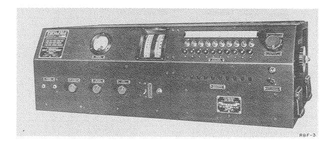
Radio Receiving Equipment RBF-3 is an f-m superheterodyne receiver designed for monitoring signals from as many as 10 sono-radio-buoy transmitting equipments. It is used in harbor defense and underwater sound detection applications.
