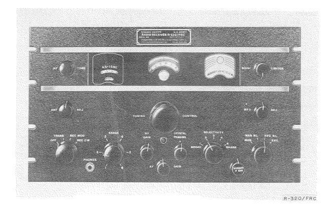
Radio Receiver R-320/FRC is an a-m (voice, cw, and mcw) receiving equipment used for general communications such as point-to-point, ground-to-air, and ship-to-shore applications or for diversity reception.
