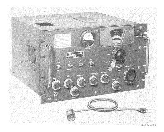
Radio Receiver R-274/FRR is a medium-, high-, and very-high-frequency a-m (voice, tone and cw) receiving equipment used for communication and special applications in fixed plant and similar installations.
