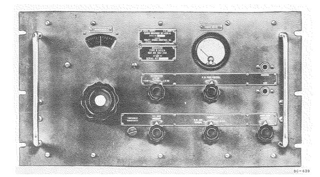
Radio Receiver BC-639 is a-m (tone, cw, and icw) receiving equipment used for ground-to-air and point-to-point communication, and in direction finding applications.
