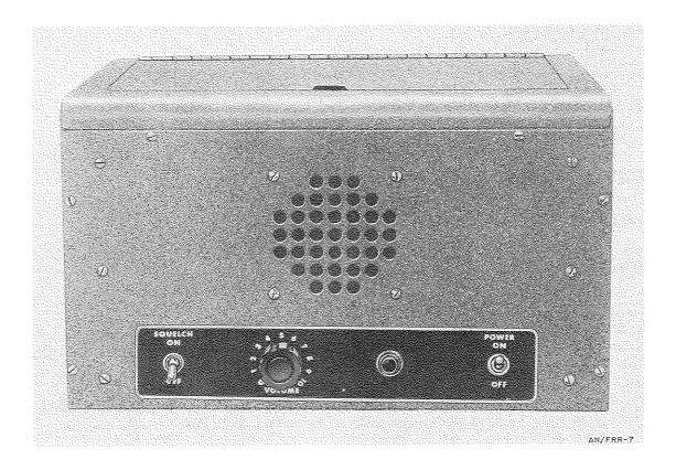
Radio Receiving Set AN/FRR-7 is a crystal-controlled, fixed-frequency, a-m (voice and tone) receiving equipment operating in the medium frequency band. It is used at army and higher head-quarters.
