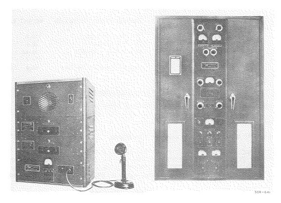
Radio Set SCR-641 is normally used for two-way radiotelephone, ground-to-air and point-to-point communication. It is ground, fixed, station equipment operated at advanced air bases for aircraft traffic control.
