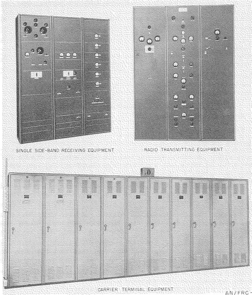
Radio Set AN/FRC-10 is a high-power, h-f, long range, a-m (voice, and tone) radioteletype communication equipment used in long distance, fixed plant applications at army, and equivalent headquarters.
