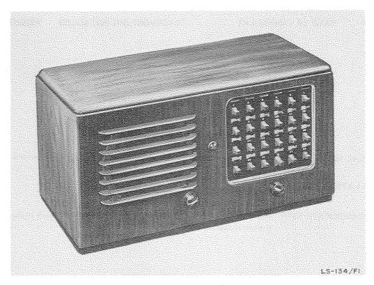
Intercommunicating Station LS-134/F1 is a master or control station unit of an intercommunication system. It is used in systems serving large headquarters buildings, depots, communications centers, or similar installations at army and higher headquarters.
