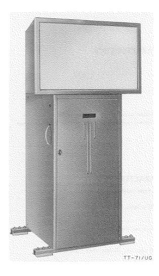
Teletypewriter Printer-Projector TT-71/UG is fixed station receiving-only equipment. It projects its received messages upon a translucent screen and is used for conference communication, group orientation and instruction, and similar applications. It is used at higher headquarters.
