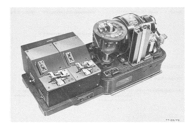
Transmitter-Distributor TT-26/FG is an automatic teletypewriter transmitting equipment which sends electrical impulses (according to the five-unit, start-stop teletypewriter code) to two lines, simultaneously from previously perforated paper tape. It is used in the communications zone of a theater of operations or in the zone of interior.
