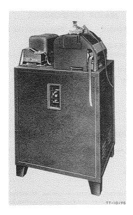
Teletypewriter TT-10/FG is an automatic sending and receiving teletypewriter station equipment used for receiving, recording, and retransmitting teletypewriter communications, by means of perforated paper tape, at corps and higher headquarters.
