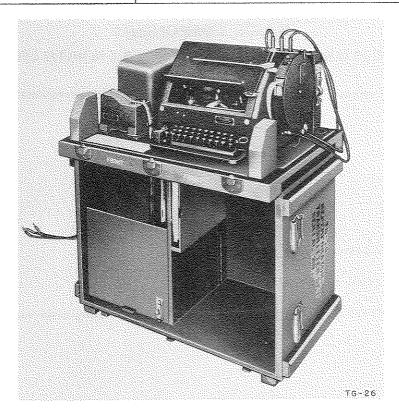
Reperforator-Transmitter TG-26 is a portable, field, teletypewriter tape relay station equipment used for the automatic (or manual) transmission, and reception of messages in the form of perforated and typed paper tape, in field wire, cable, or open wire systems serving division and higher headquarters.
