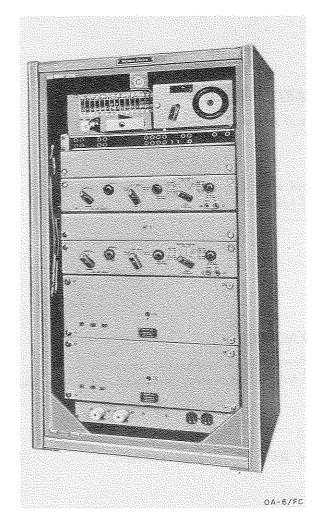
Telegraph Repeater OA-6/FC is a packaged, d-c repeater equipment, used to extend the operating range of telegraph systems used for teletypewriter communication over composited open wire, or simplexed open wire or cable facilities serving army and higher levels.
