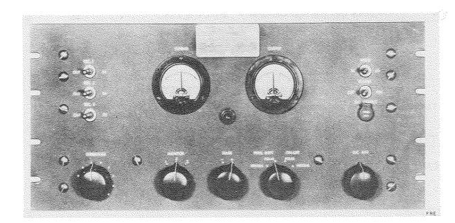
Frequency Shift Receiver Converter Equipment FRE is designed to adapt Navy Model Diversity Radio Receiving Equipment RDM for reception of frequency-shift-keyed signals. It is used with associated equipment to provide ship-to-shore and point-to-point radiotelegraph or radioteletype reception.
