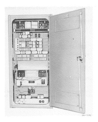
Telephone Repeater OA-7/FC is a v-f telephone equipment used to extend the operating range of 2- or 4-wire telephone systems operating over open wire or cable and serving army or equivalent headquarters.
