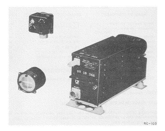
Radio Receiving Equipment RC-103 consists of an airborne receiver with six preset crystal-controlled channels, used for receiving signals transmitted by Army Air Force Instrument Approach System (formerly known as Instrument Landing System SCS-51). It is normally operated by means of a radio control box which provides ON/OFF, volume control, and frequency selection.
