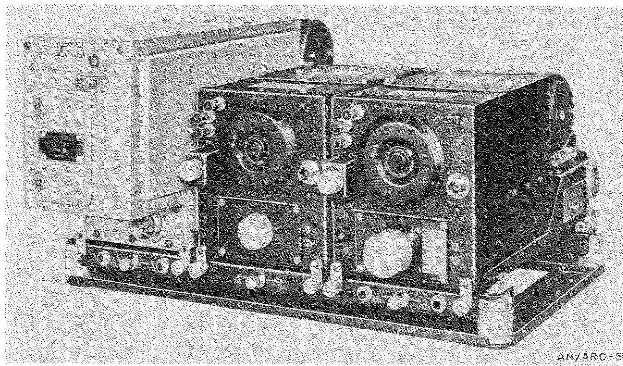
**Radio Equipment AN/ARC-5** is a multichannel I-f, m-f, h-f and v-h-f, am (cw, mcw, voice) transmitting and receiving equipment assemblage for installation in aircraft for general air-to-ground communication, and for reception of instrument landing and navigational signals. It is a multiple-unit equipment, the number of transmitters and receivers employed (limit of five receivers and eight transmitters) depend upon the type of installation.
