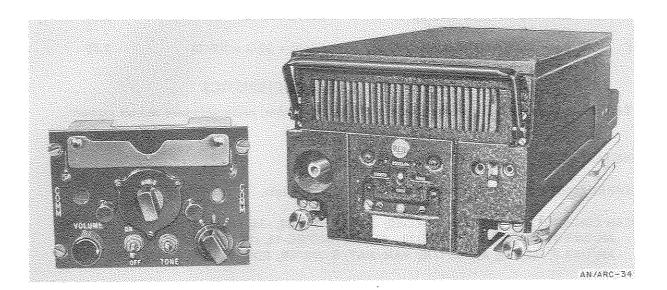
Radio Set AN/ARC-34 is a miniaturized version of Radio Set AN/ARC-33. It is an airborne, combination transmitter—receiver unit for two-way, air-to-air, and air-to-ground communication in the u-h-f range 225.0 to 399.9 mc.
