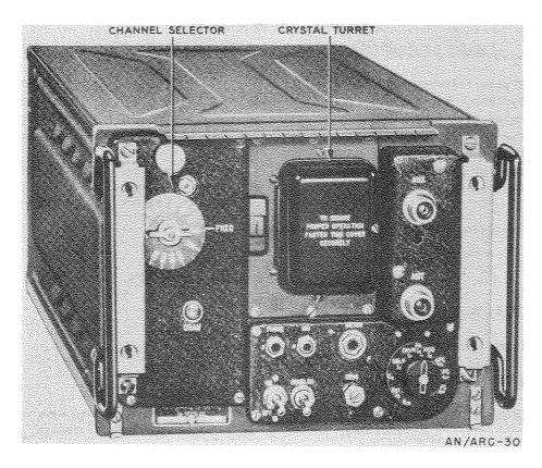
Radio Set AN/ARC -30 is an airborne v-h-f and u-h-f automatic relay station equipment for extending the range of a-m (voice) radio communication between a ship or shore station and a second aircraft in flight. The transmitted signal from a ship or shore station is received by one transceiver, and applied through a relay unit to the second transceiver for relaying to the aircraft with which contact is desired.
