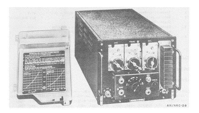
Radio Set AN/ARC-28 is an airborne v-h-f automatic relay station equipment for extending the range of a-m (voice) radio communication between a shore station, or ship, and other aircraft. A transmitted signal from a ship or shore station is received by one transceiver, and applied through a relay unit to the second transceiver for relaying to the aircraft with which contact is desired.
