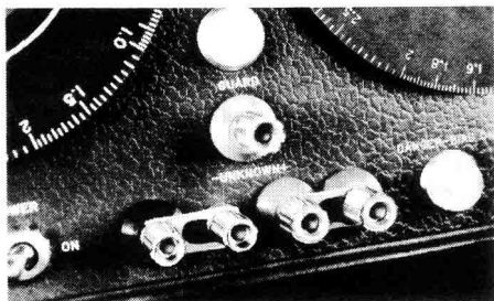
Figure 3-1. UNKNOWN and GUARD terminals on the bridge.
