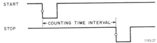
Figure 3-4 Time-interval measurement start and stop pulses.
